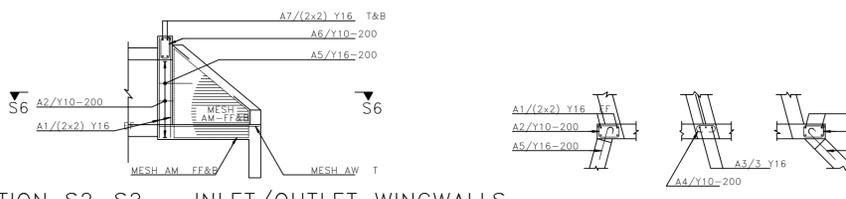
SECTION S2-S2 – INLET/OUTLET WINGWALLS HEADWALL & WINGWALLS – REINFORCEMENT
